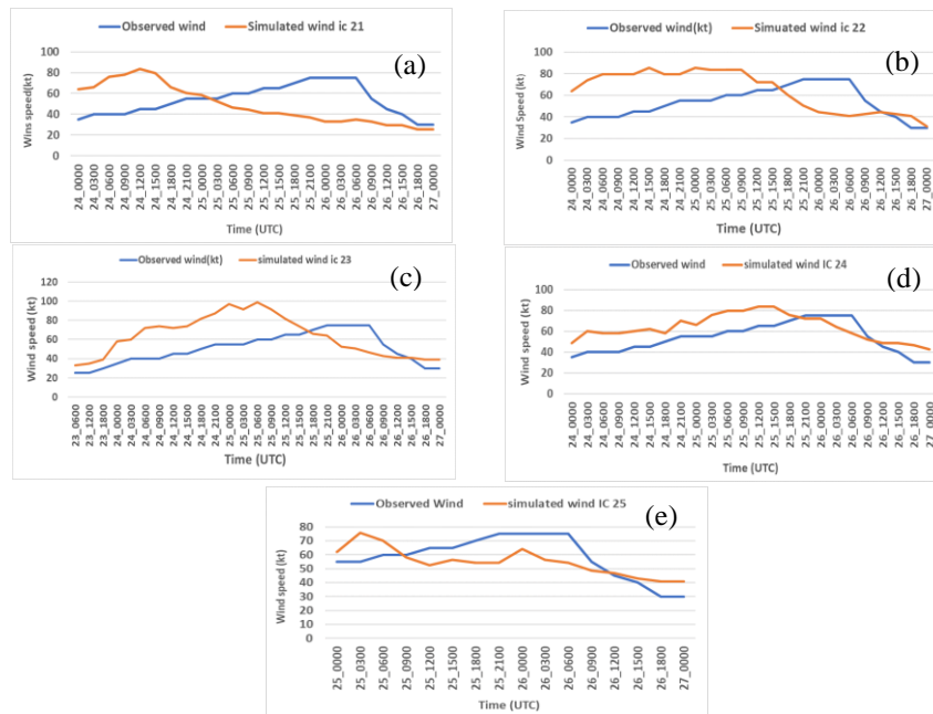
Figure 4: Comparison of model simulated wind speed (kt) with the observed speed for (a) 144 hours run (b) 120 hours run (c) 96 hours run (d) 72 hours run (e) 48 hours run respectively.
